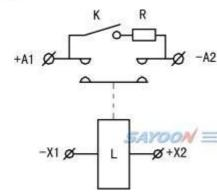
Single Pole Single Throv Contactor. (One Normal Open) +A1.-A2 Main Contact Terminal
